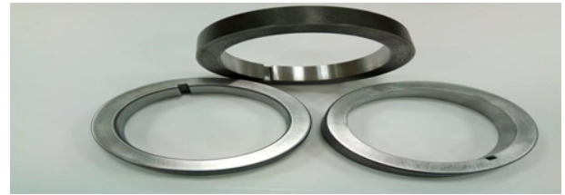
Figure 1: Rings of material C 60 (DIN), with hardness 60 \pm 2 HRC
