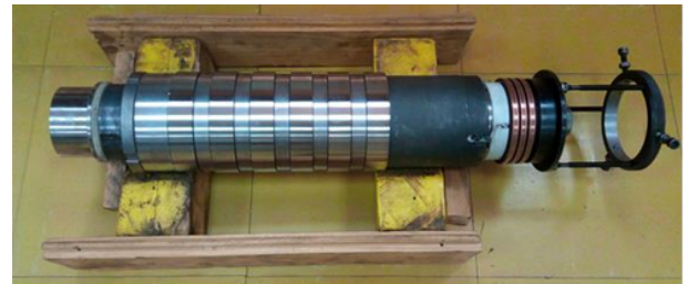
Figure 2: Special aid for the investigation of the average temperature in the cutting process during turning
